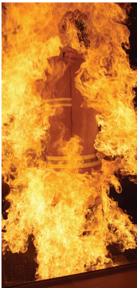
The eight second burn test was undertaken on the 2006 version of the male heat sensing manikin known as RALPH
